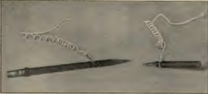
FIG. 132. Pencils ready for making an arc light.
